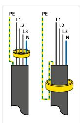
Never pass a PE conductor through the measuring current transformer
