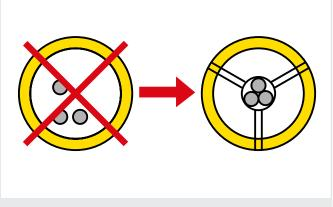
The leads must be aligned with the centre of the measuring current transformer
