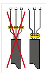
Make sure that all currentcarrying leads are passed through the measuring current transformer
