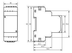
Figure: Dimension diagram (in mm)
