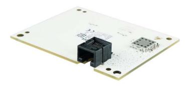
For use in combination with charge controllers used in electric vehicle charging stations, wall boxes and street light charging points
